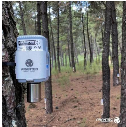
Figure 1: Standardized wireless sensor node (Arantec monitoring unit) deployed in a forest environment for real-time environmental monitoring and early wildfire detection.
