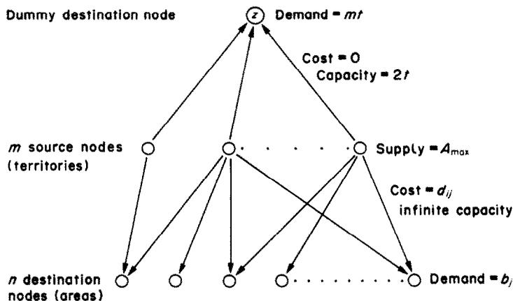
Fig. 1. Network formulation of the capacitated transportation problem (4.5).
