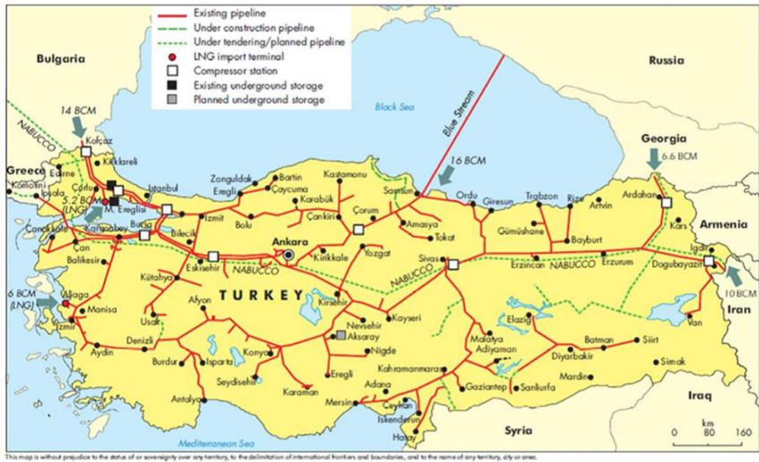
Figure 5.5. Pipeline System in Turkey [53]
