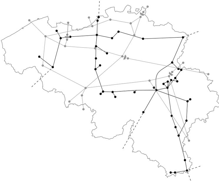
Figure 7.1: The high-voltage Belgian electrical power grid (black) and high-pressure gas network (gray). Note that the indicated connections do not represent the actual physical line paths.
