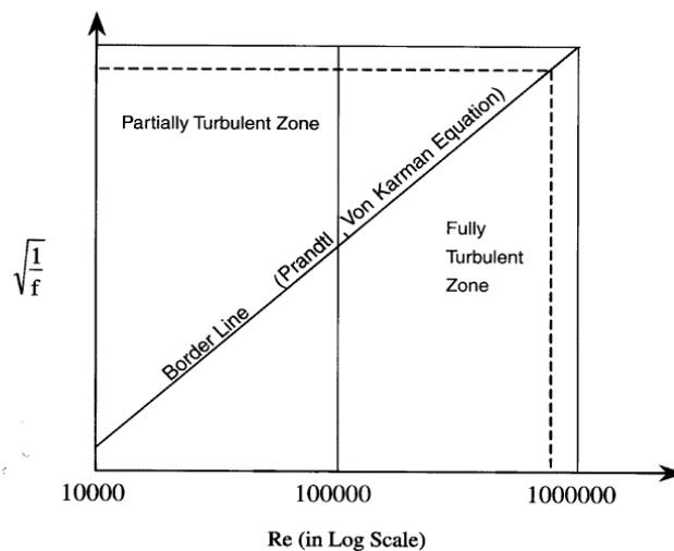
Fig 3. Representation of fully turbulent/partially turbulent zones by the Prandtl- Von Karman Equation [11]
