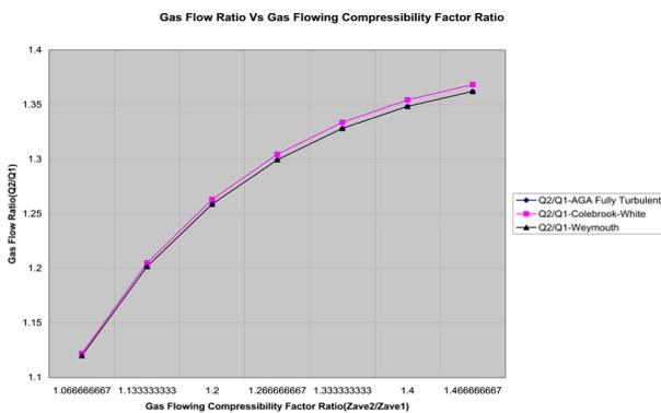
Fig 13. The impact of gas flowing compressibility factor ratio change on gas flow ratio
