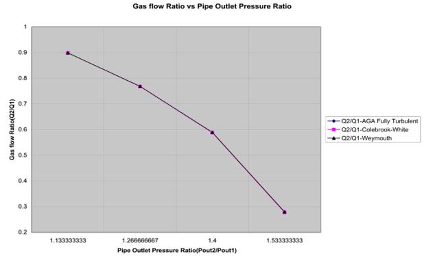
Fig 9. The impact of pipe outlet pressure ratio change on gas flow ratio
