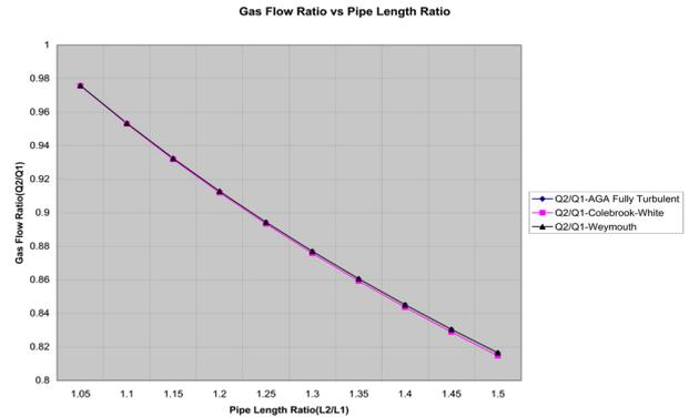
Fig 5. The impact of pipe length ratio change on gas flow ratio
