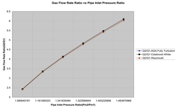
Fig 8. The impact of gas pipe inlet pressure ratio on gas flow ratio
