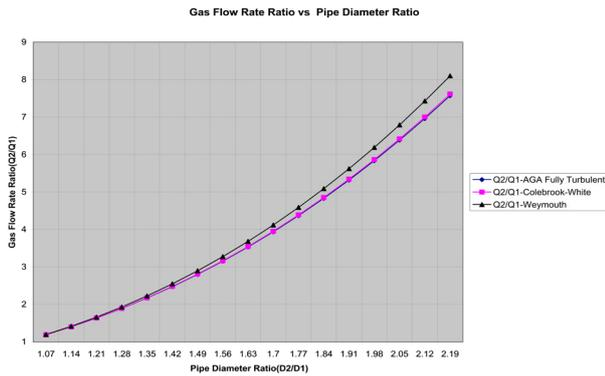
Fig 4. The impact of pipe diameter ratio change on gas flow ratio
