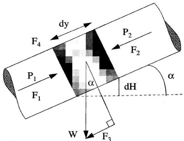
Fig 2. Demonstration of all forces acting on a gas particle moving in a non-horizontal pipeline[10]
