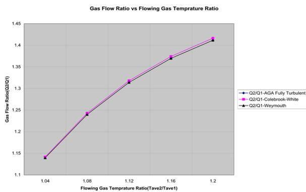
Fig 10. The impact of flowing gas temperature ratio change on gas flow ratio
