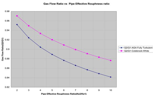
Fig 6. The impact of pipe effective roughness ratio change on gas flow ratio
