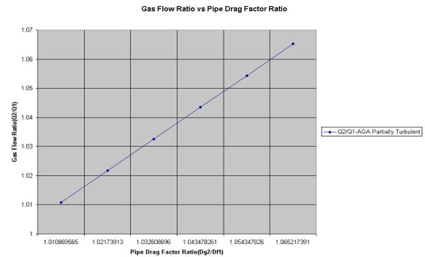
Fig 7. The impact of pipe drag factor ratio change on gas flow ratio
