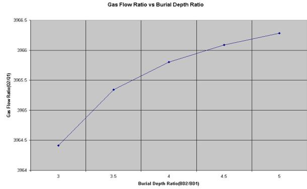
Fig 16. : The impact of burial depth change on gas flow ratio
