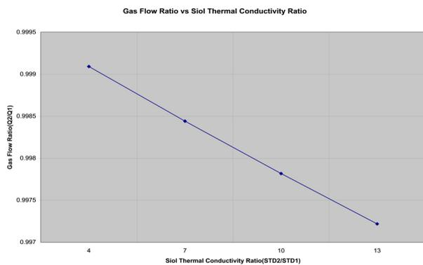
Fig 17. The impact of soil thermal conductivity ratio change on gas flow ratio
