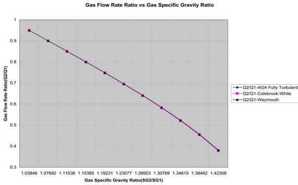
Fig 12. The impact of gas gravity ratio change on gas flow ratio
