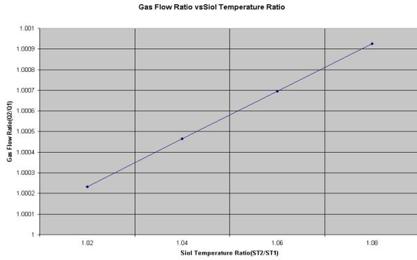
Fig 15. The impact of soil temperature ratio change on gas flow ratio
