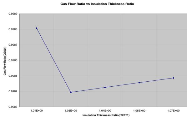
Fig 19. The impact of insulation thermal conductivity ratio change on gas flow ratio
