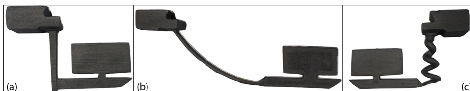
Fig. 9. 17-4 stainless steel alloy castings featuring (a) straight sprue (b) parabolic sprue casting (PSC)(c) conical-helix sprue casting (CHSC).
