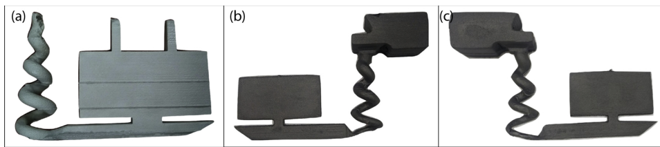
Fig. 24. Demonstrating manufacturability of optimized conical-helix sprues for (a) Aluminum 319 alloy (b) 17-4 stainless steel alloy (c) Class 30 Gy Cast Iron.
