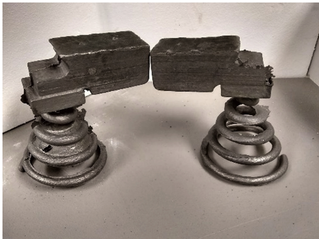
Fig. 22. Fluidity spiral test using sprue optimization and 3DSP mold.
