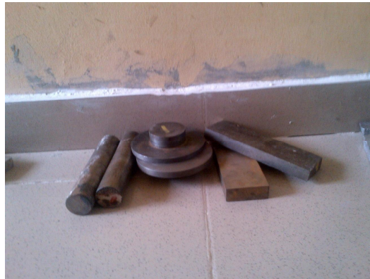
Fig. 12. Slightly machined grey cast iron components
