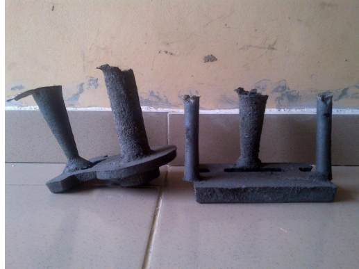
Fig. 11. As-cast components in grey cast iron
