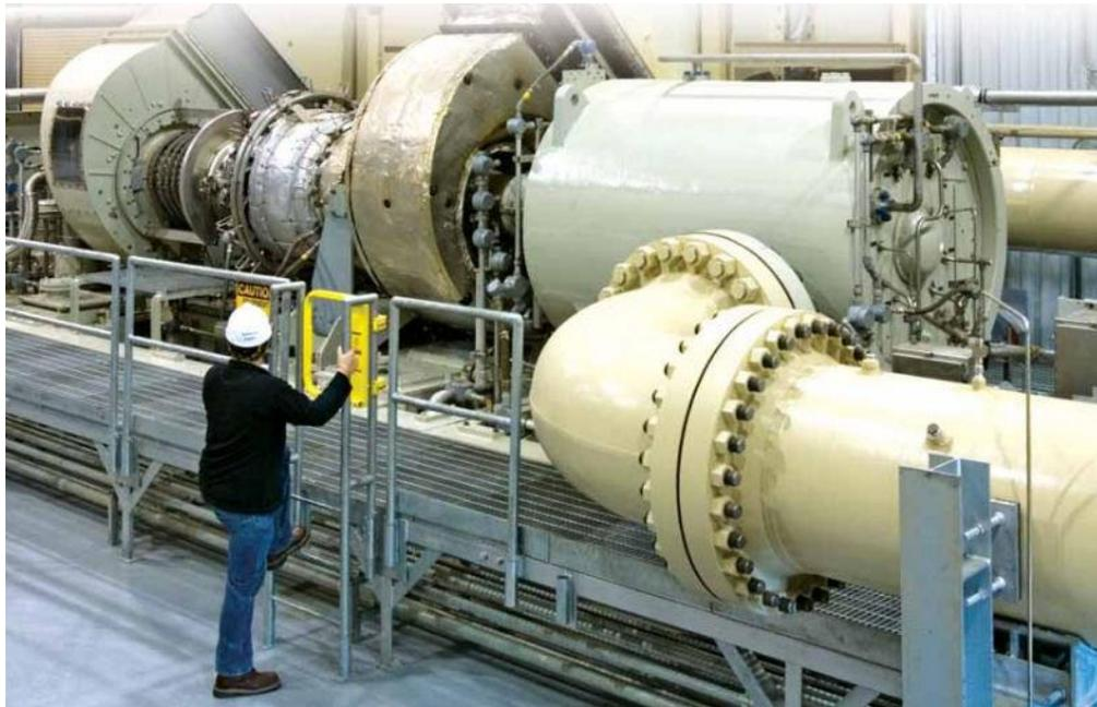
Figure 9: Centrifugal gas compressor. Source: Caterpillar Company (2016)
