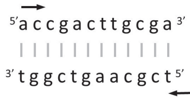
Figure 6. An example of the reverse and complementary sequence. A DNA sequence is always read from 5' end to 3' end. Due to the complementarity rule, A on one strand is connected with T on the other, and G is connected with C. The following fragment of the DNA helix can be read as 'accgacttgca' or 'tcgcaagtcgg'.
