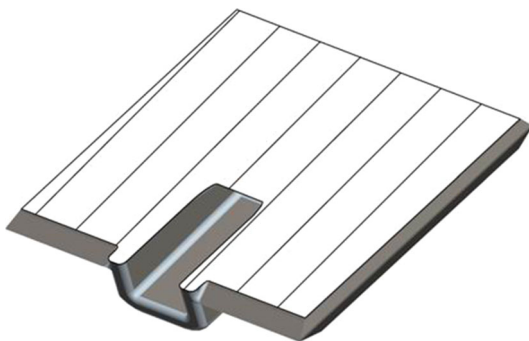
Figure 4. Area cross section of casting part A_i (52 mm) = 78,041.27 mm 2 .
