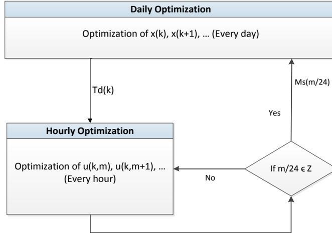
Figure 3.3: Upper and Lower layer optimizations of multi-layer MPC
