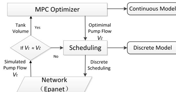
Figure 5.2: Two-layer Control Scheme
