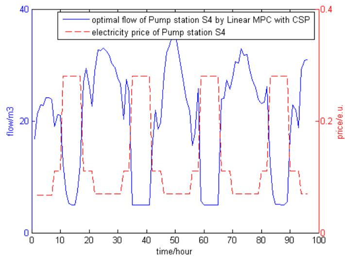
Figure 4.22: Comparison between pump flow and its electricity price
