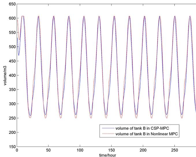
Figure 4.13: Comparison of water evolution in tank between CSP-MPC and non-linear MPC
