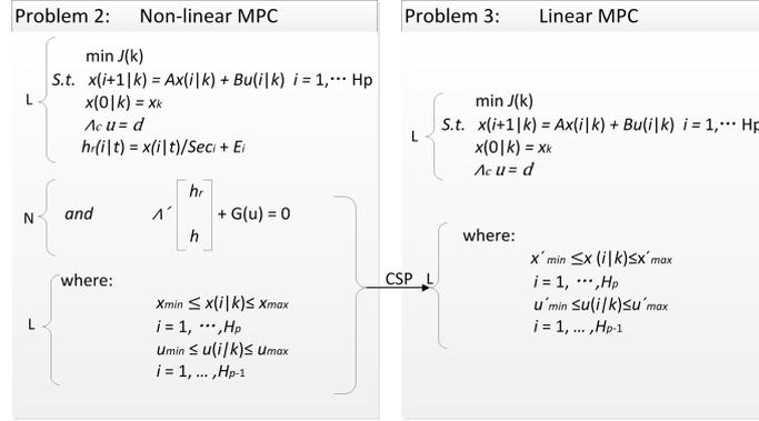
Figure 4.2: Working principle of CSP-MPC
