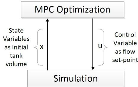
Figure 3.13: Feedback structure of Simulation and Optimization
