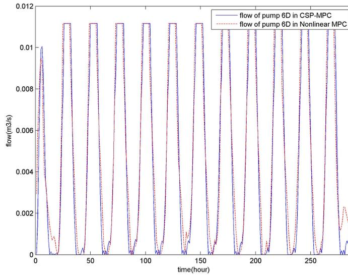
Figure 4.14: Comparison of pump flow between CSP-MPC and Non-linear MPC
