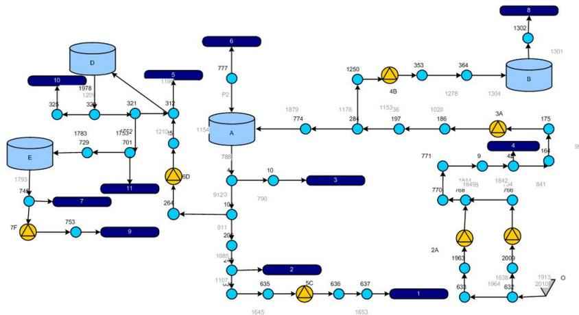
Figure 4.12: The PLIO model of Richmond water distribution network
