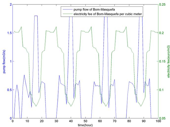
Figure 3.7: Pump flow with electricity price
