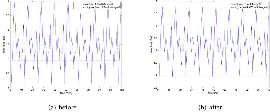
Figure 3.5: River flow comparing with ecological level before and after ecological control in river Llobregat
