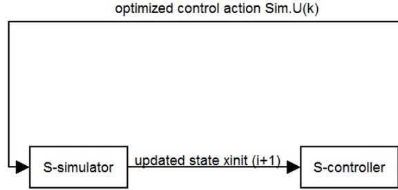
Figure 3.15: Integration of optimization and simulation blocks
