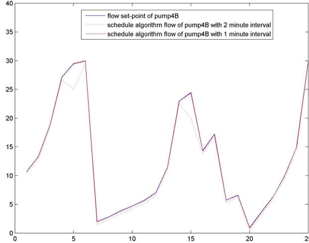
Figure 5.4: Flow errors in different time intervals
