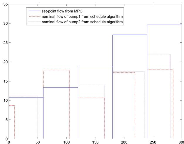
Figure 5.3: Optimal Schedule for Pump4B with two pump branches
