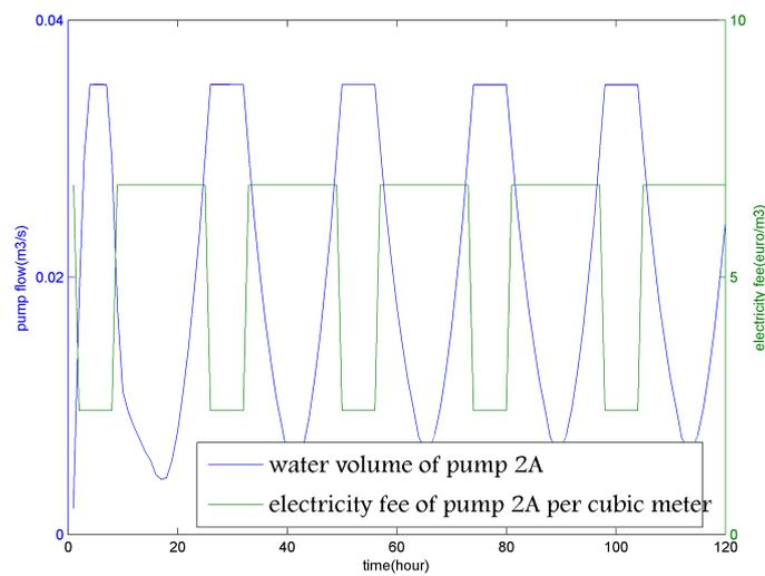
Figure 4.9: Comparison between pump flow and its electricity price
