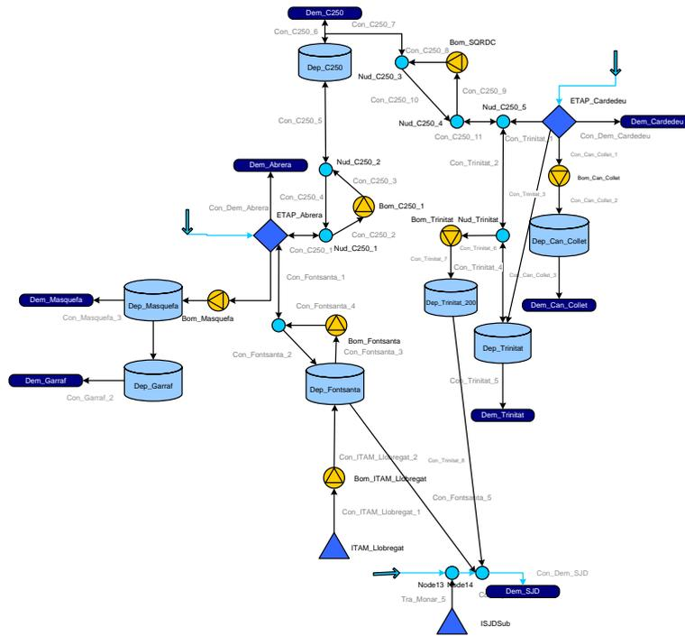
Figure 1.5: Aggregate transportation layer of Catalunya Regional Water Network
