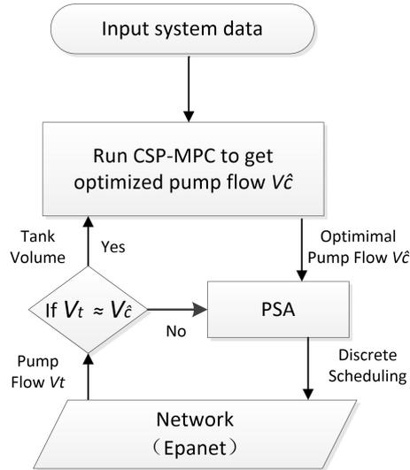
Figure 4.3: Simulating CSP-MPC using Epanet
