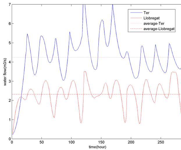
Figure 3.11: Flows from two rivers after using temporal coordination with  $x$ -time and  $y$ -flow axis
