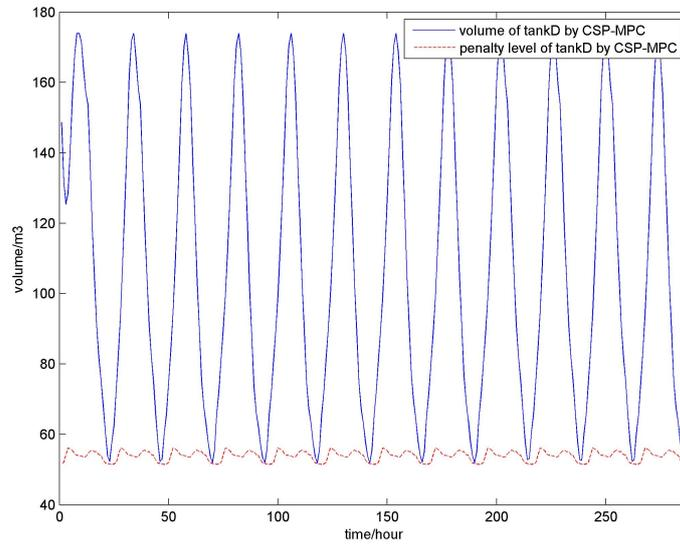
Figure 4.8: Comparison between tank penalty by CSP and its volume evolution
