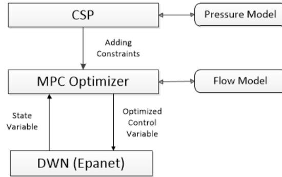
Figure 4.1: The multi-layer control scheme
