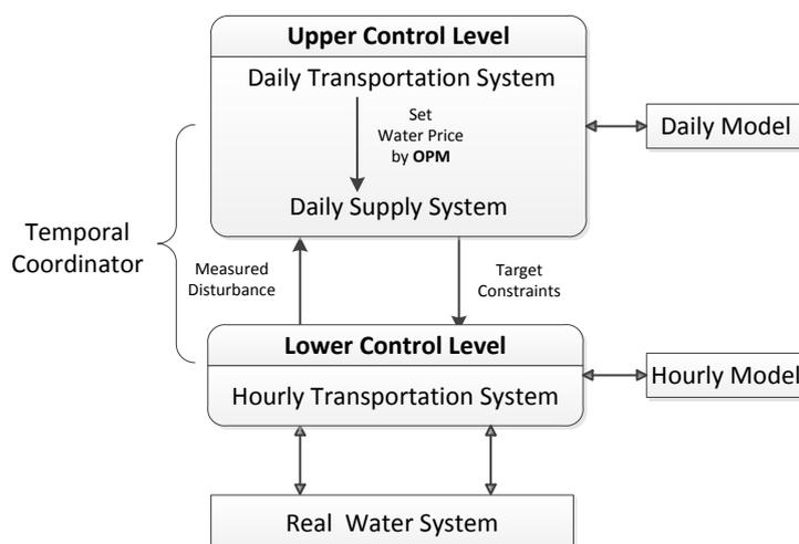
Figure 3.1: Temporal hierarchical coordinating structure
