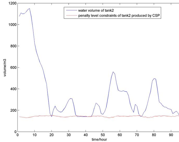
Figure 4.21: Comparison of tank volume and the safety volume by CSP-MPC
