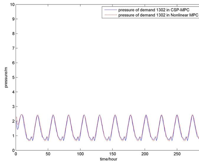
Figure 4.15: Comparison of demand node pressure between CSP-MPC and Non-linear MPC
