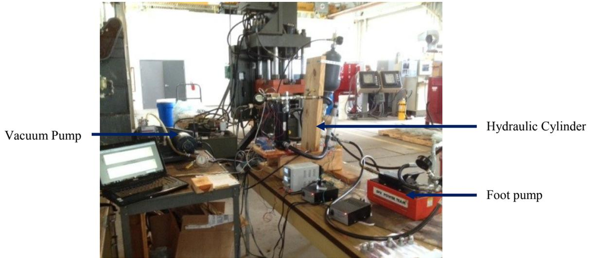
Figure 3.4 Bench test setup
