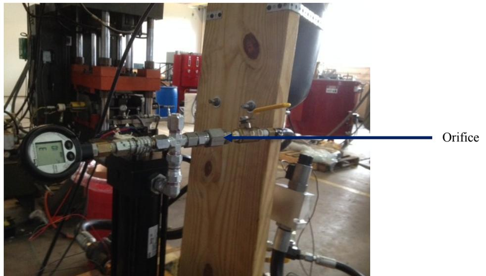
Figure 3.5 Orifice setup
