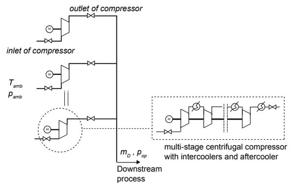
Fig. 1. Compressor station with multi-stage centrifugal compressors in parallel.
