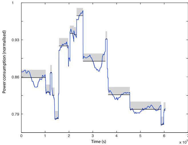
Fig. 7. steady-states of operation from the steady-state detection algorithm.
