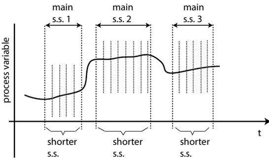
Fig. 4. Main and shorter steady-states of a process variable.
