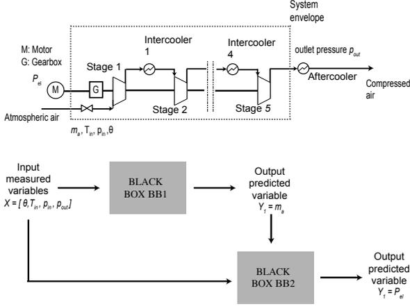
Fig. 5. Regression models of a multi-stage compressor.
