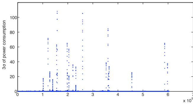
Fig. 8.  $3\sigma$  of the power per data set window of the fourth compressor during step tests.
