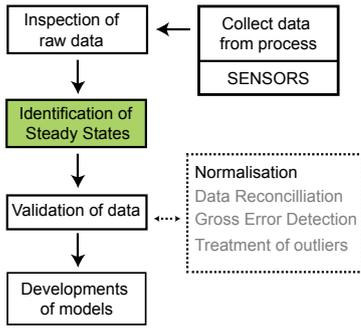
Fig. 2. Typical procedure to process raw data for developing data-driven models.
