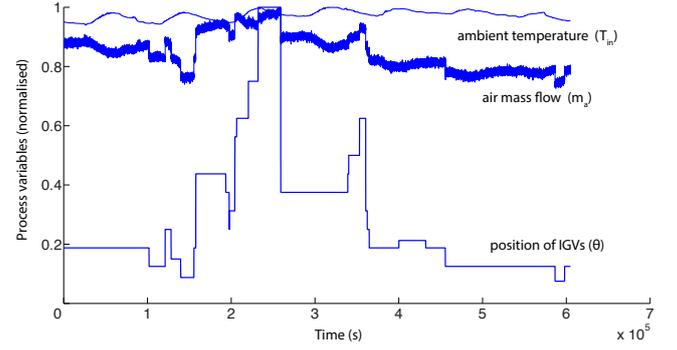
Fig. 6. Several process variables of the operation of an industrial centrifugal compressor over time.
