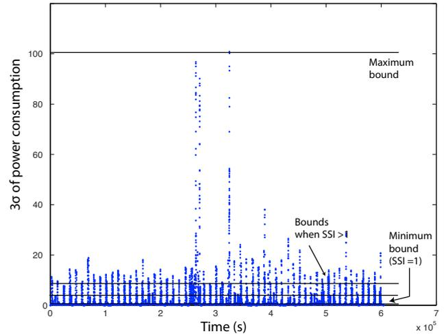
Fig. 9.  $3\sigma$  of power per data set window of compressor 1.
