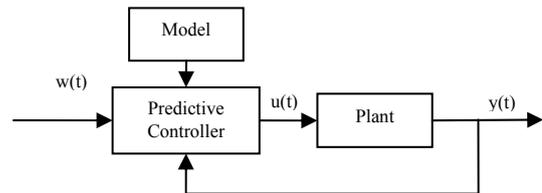
Figure 3: The Concept of Model-based Predictive Control
