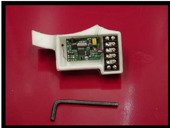
Figure 5-19. CTS Breadboard in Housing
