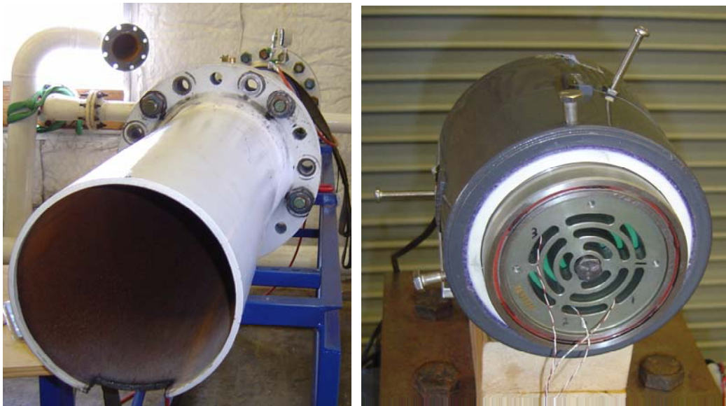
Figure 4-18. Burst-Membrane Shock-Tube (Left) and Instrumented Valve Fixture (Right)
