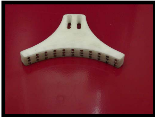
Figure 5-18. Magnet Array for RCTF Testing
