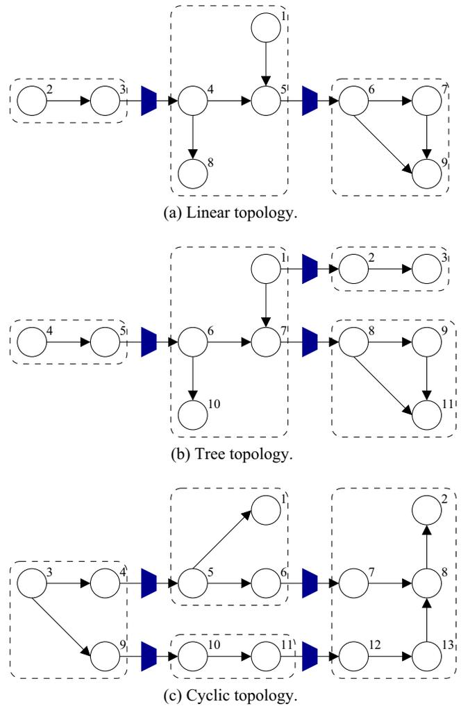
Fig. 8. Different kinds of pipeline network topologies.
